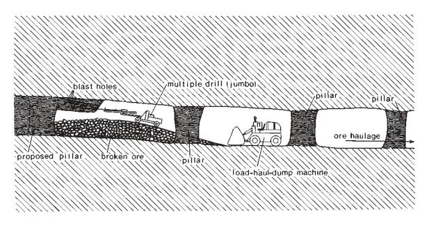
Figure 16.—Room and pillar mining method.
