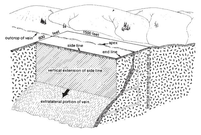
Figure 2.—Extralateral rights of a lode mining claim.
