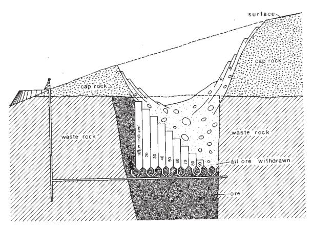
Figure 20.—Block caving underground.
