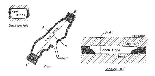
Figure 15.—Open stope mining method.
