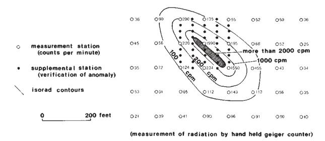
Figure 11.—Plan showing gamma radiation over a uranium ore body.
