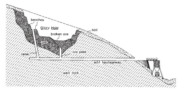
Figure 21.—The glory hole mining method.
