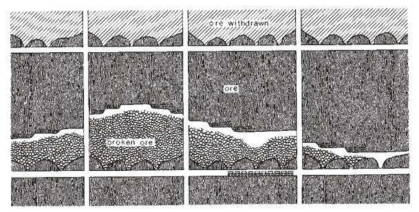
Figure 17.—Shrinkage stoping.
