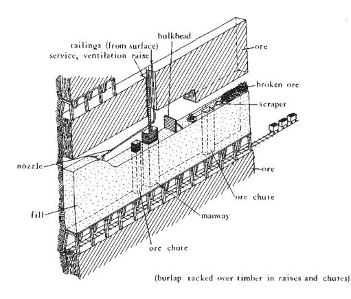
Figure 18.—Hydraulic stope fill.
