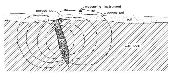
(Measurement of electric current spontaneously generated by a sulphide body)
