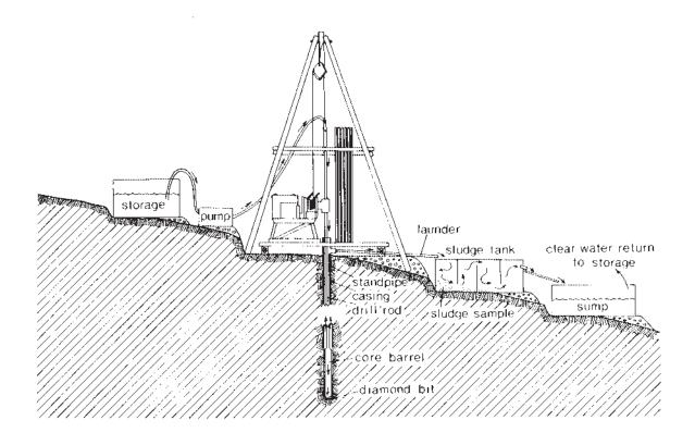
Figure 12.—Diamond drilling, collection of sludge samples.
