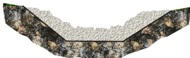
Cross Section of an Open Limestone Channel
